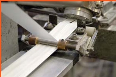
In-line adhesive application
