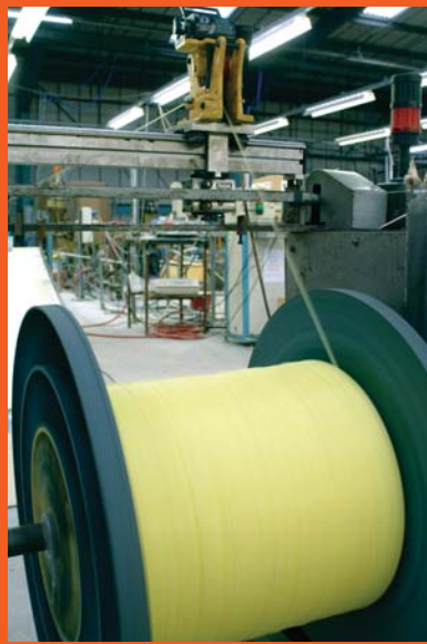
Cable filler spooling
